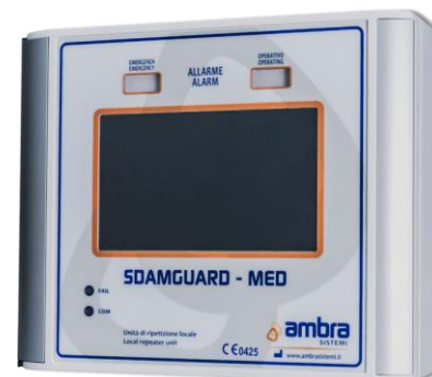
Local repeater for networks constituted by SDAM-MED and/or SDAL-MED
