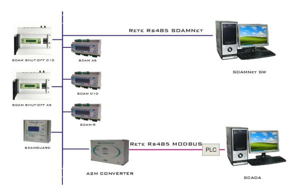
**A2M Converter** module allows interfacing the local monitoring network SDAMNet for pure, technical and non-flammable gases to the **mainframe** system based on PLC and/or SCADA systems, normally used in the control rooms, by a Modbus gateway.
