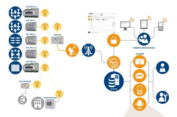
The server CrioSystemSupervisor (CSS) allows remote monitoring of the **SDAMNet Plus** units. The client CSS user interface is available on the web for PC, smartphone or tablet by WebAPP, without any download or user-level installation.
